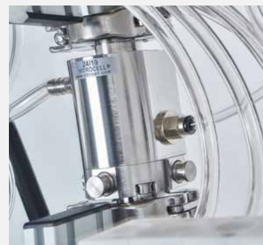
Dynamic dilution system with air jets featuring a constant flow rate over the entire system.
