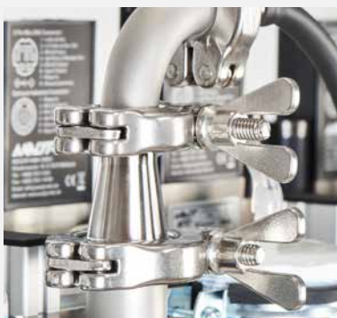
Small flange connections for easy disassembly and cleaning.
