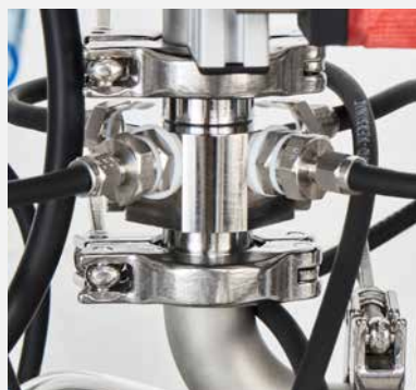
Isokinetic Sampling probes made of stainless steel.
