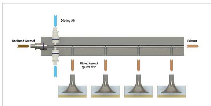
Image 1. Dilution schematic of Vitrocell® 24/4 module.
