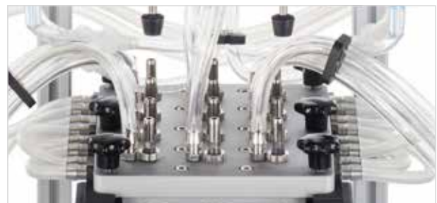
VITROCELL® 12/12 quick connect system replaces the mounting of tubing material.
