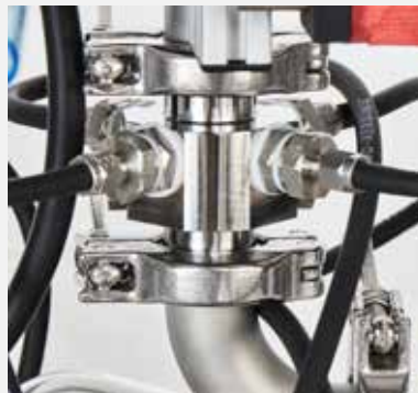
Isokinetic Sampling probes made of stainless steel.
