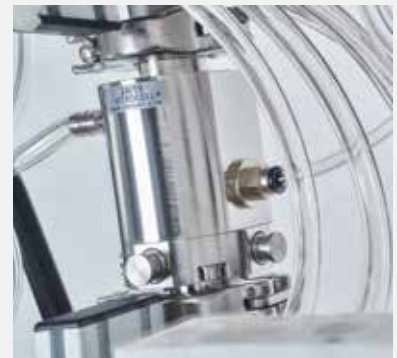
Dynamic dilution system with air jets featuring a constant flow rate over the entire system.
