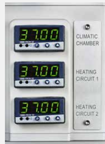
Heating Systems for base module and climatic chamber to avoid effects of aerosol condensation.
