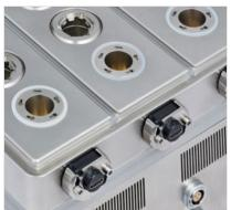
The sQCM 12 sensor (left) can be fitted in all rows of the Cloud Alpha TRIO exposure module (right).
