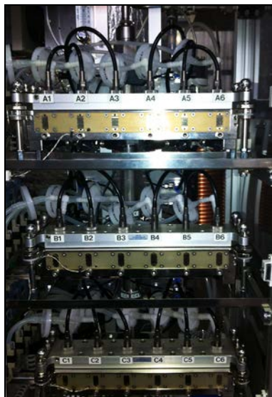
HICE exposure unit using 3 VITROCELL® 6/6 exposure modules. The unit was built by KIT Karlsruhe for the HICE project.
