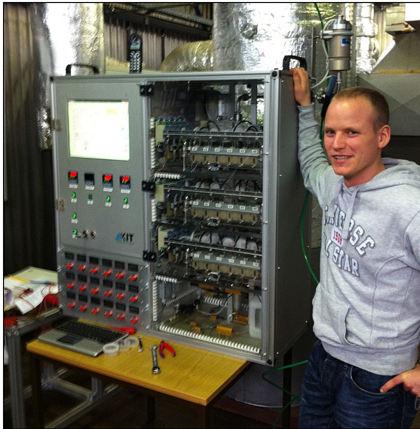
HICE exposure unit using 3 VITROCELL® 6/6 exposure modules. The unit was built by KIT Karlsruhe for the HICE project.
