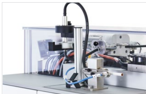
VITROCELL® Photometer connected to a VC 1 Smoking Machine.
