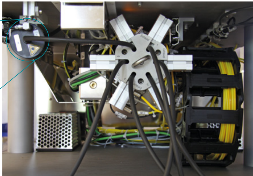
VITROCELL® VC 10 S-TYPE with VITROCELL® Particle Photometer for online particle delivery monitoring.
