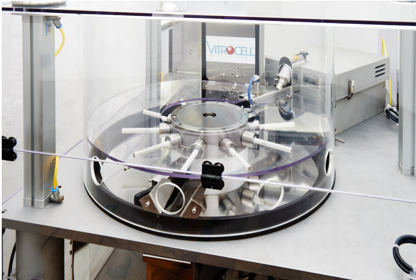
Universal smoking robot for combustion and e-cigarettes
