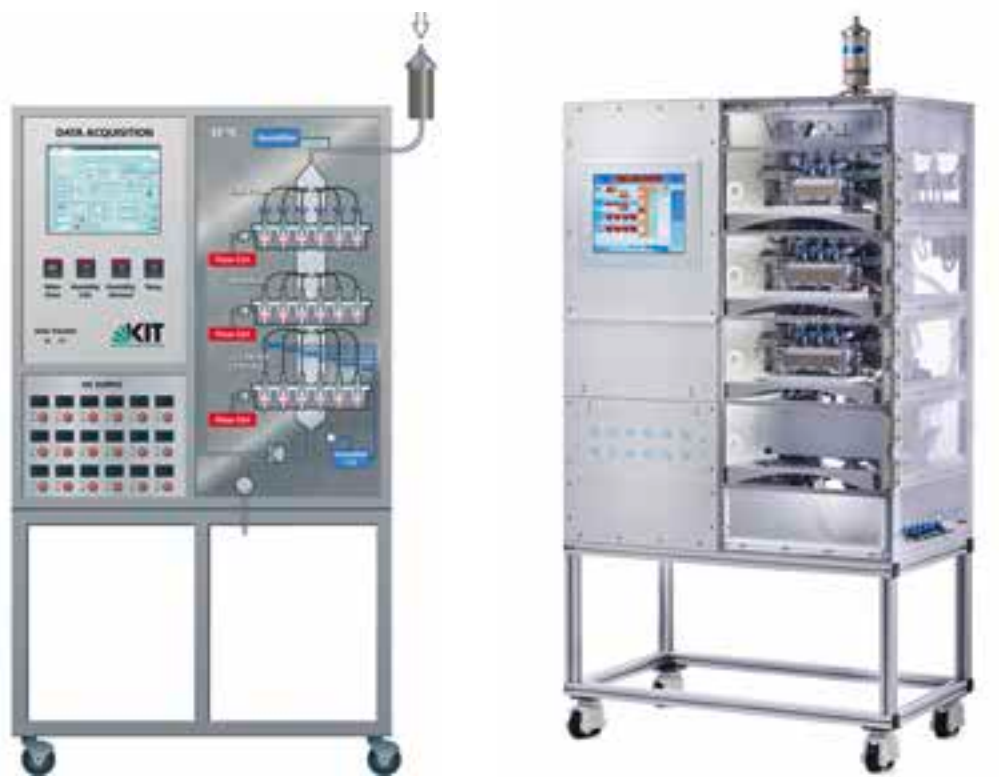
Fig. 2 Automated exposure system for reproducible exposure of bioassays at the air-liquid interface. Left: Schematic view of the main process components. Right: Photograph of Vitrocell system.
