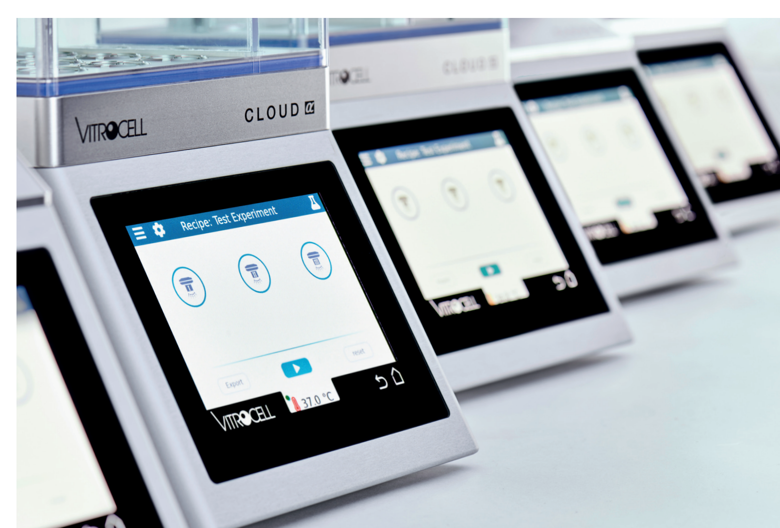
Fig. 6: Touchscreen control of VITROCELL® Cloud Alpha devices
