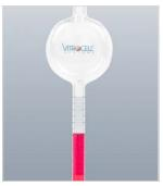
The drop of fluid in mm/60 s from the setpoint mark indicates the leakage rate.
