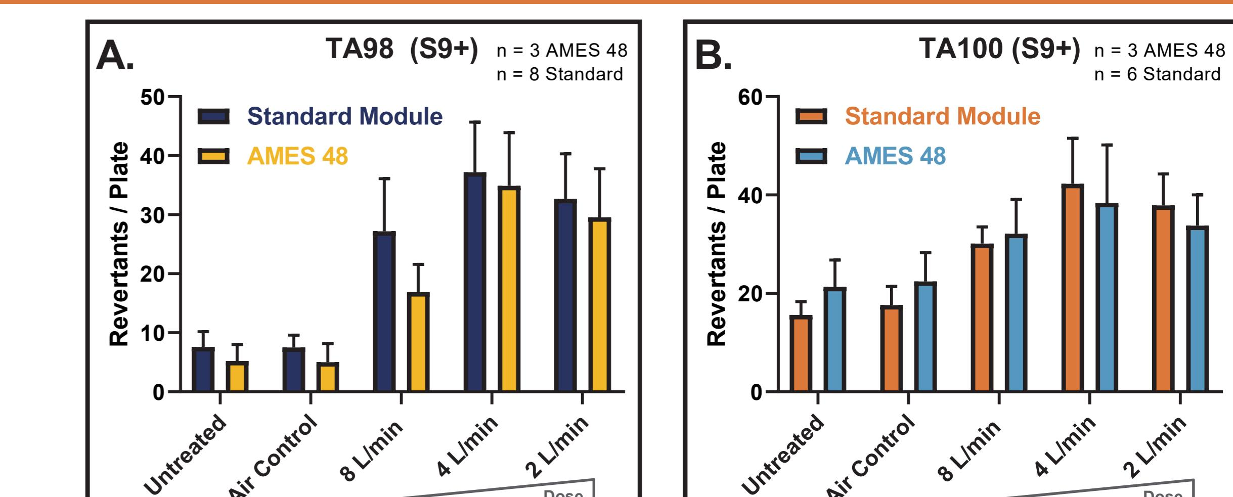
**Figure 6:** 3R4F whole smoke Ames Assay: Standard vs. AMES 48 Modules. TA98 (A) and TA100 (B) were exposed to 3R4F whole smoke generated under ISO conditions from 8 cigarettes. Standard module data taken from historical data. Revertant counts compared at equivalent dilution air flows.
