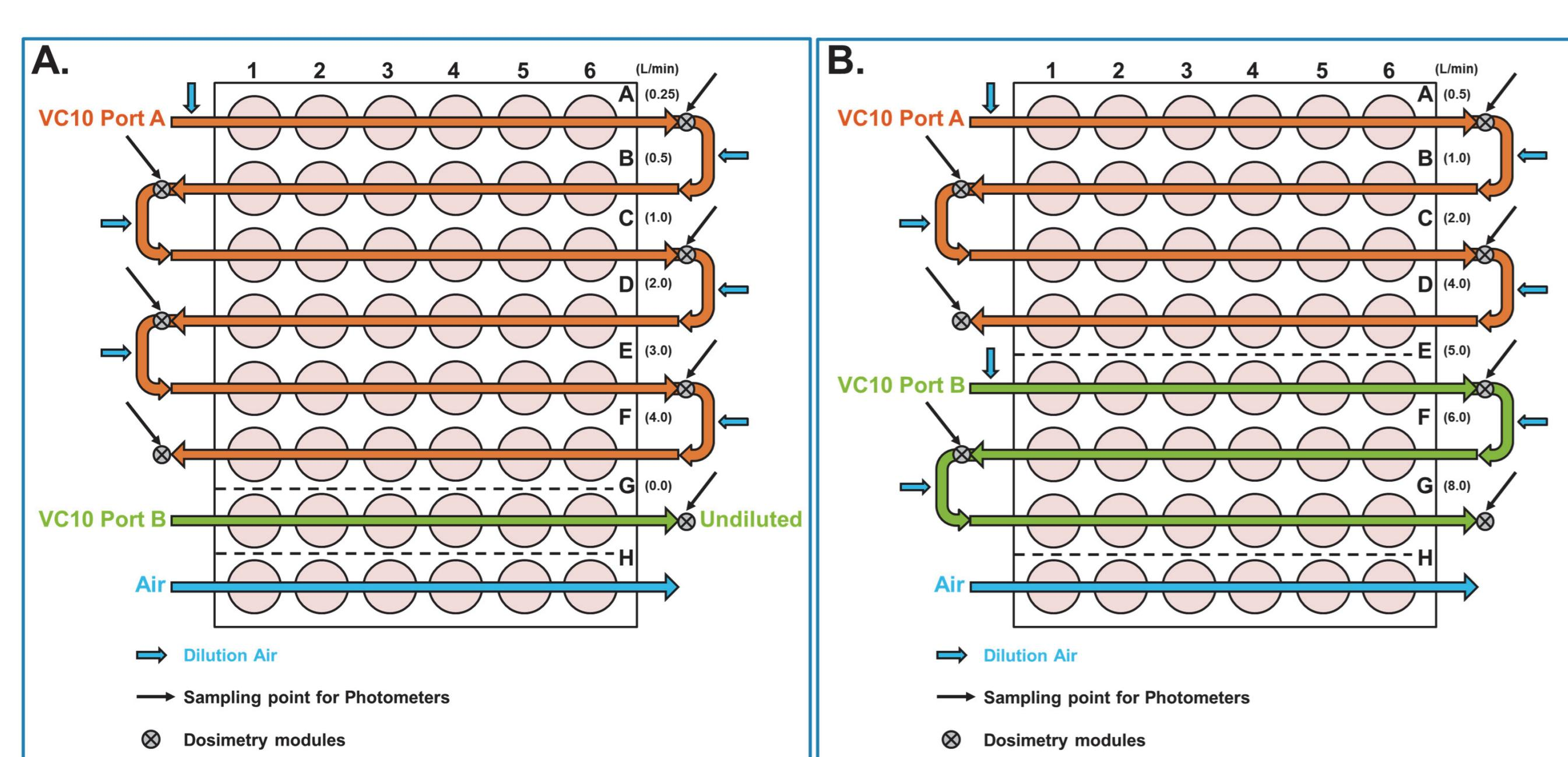
**Figure 1:** Vitrocell® Ames 48 high throughput exposure module set-up for either THP and ENDS (A) or 3R4F combustible cigarette (B). Diagrams indicate placement of photometers (—), dosimetry modules (◎) and addition of air for smoke/aerosol dilution (→).
