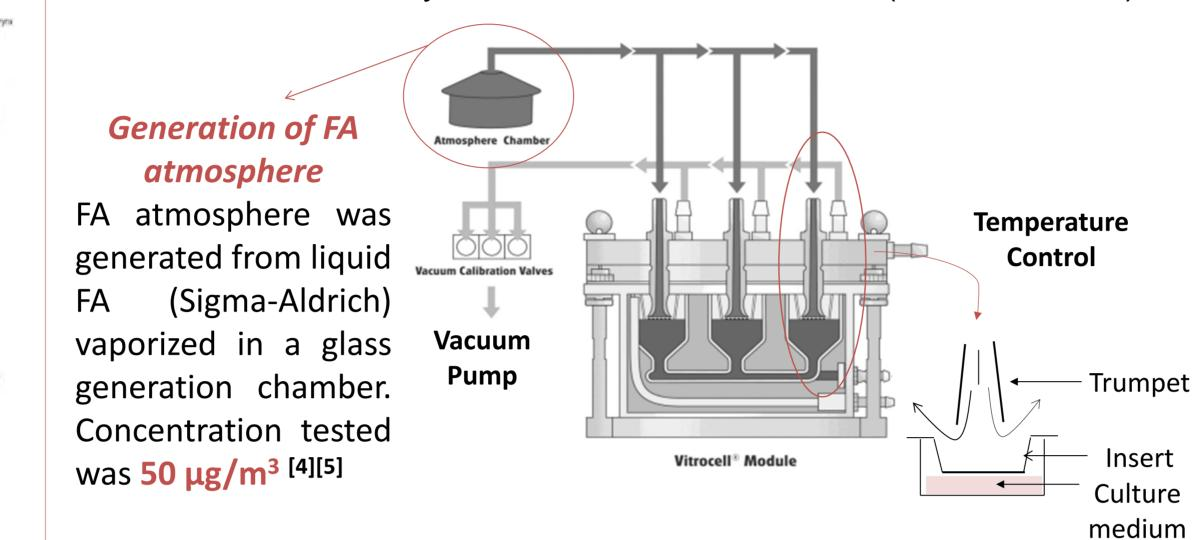
• Air-liquid exposure is performed using a trumpet device, allowing a direct contact between cells and tested atmosphere
