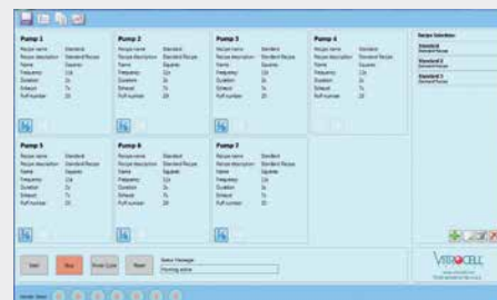
Individual program settings can be allocated to each syringe drive
