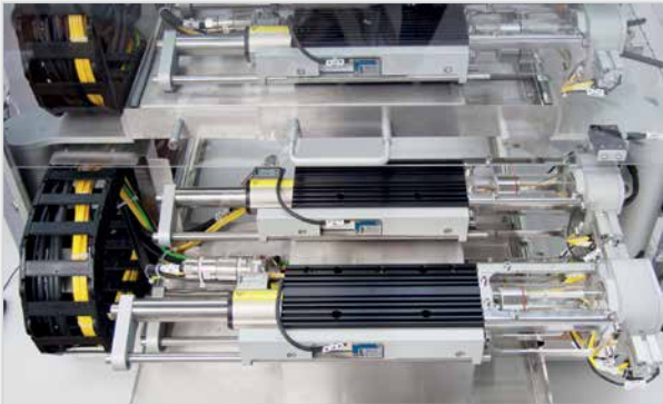
Drawer with linear motor drives
