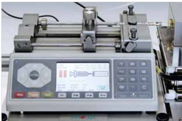
Syringe drive High precision and electronically controlled
