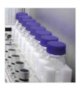
1 | Receptor fluid is stored in glass bottles and can be supplied gravimetrically or by syringe to the VITROCELL® Skin Exposure Module.
