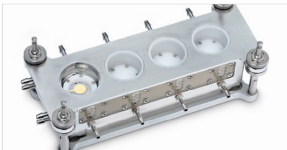
VITROCELL® AMES 4 with integrated microbalance sensor
