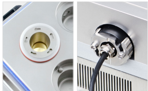
sQCM mounted in VITROCELL® Cloud Alpha 12 module (left) and the new designed oscillator (right).
