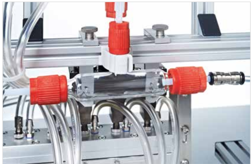
Distribution system for clean air
