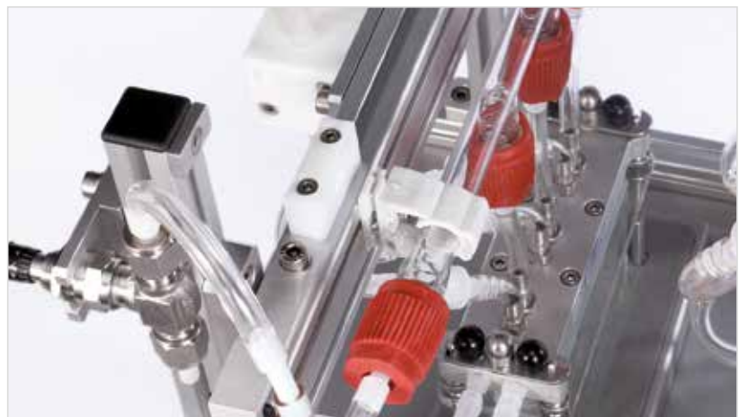
Distribution system for gaseous test substances
