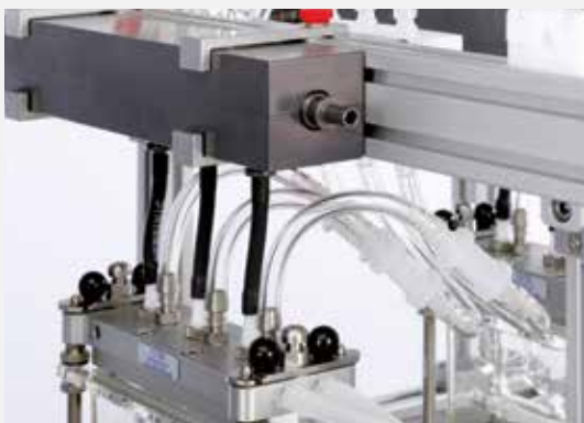
Connection of the special dilution system to the VITROCELL® 12 module
