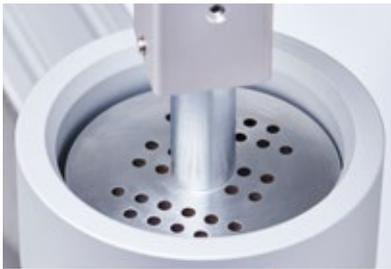
Integrated electrical heating device
