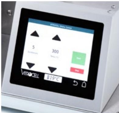
Controller for electrical heating with touchscreen display
