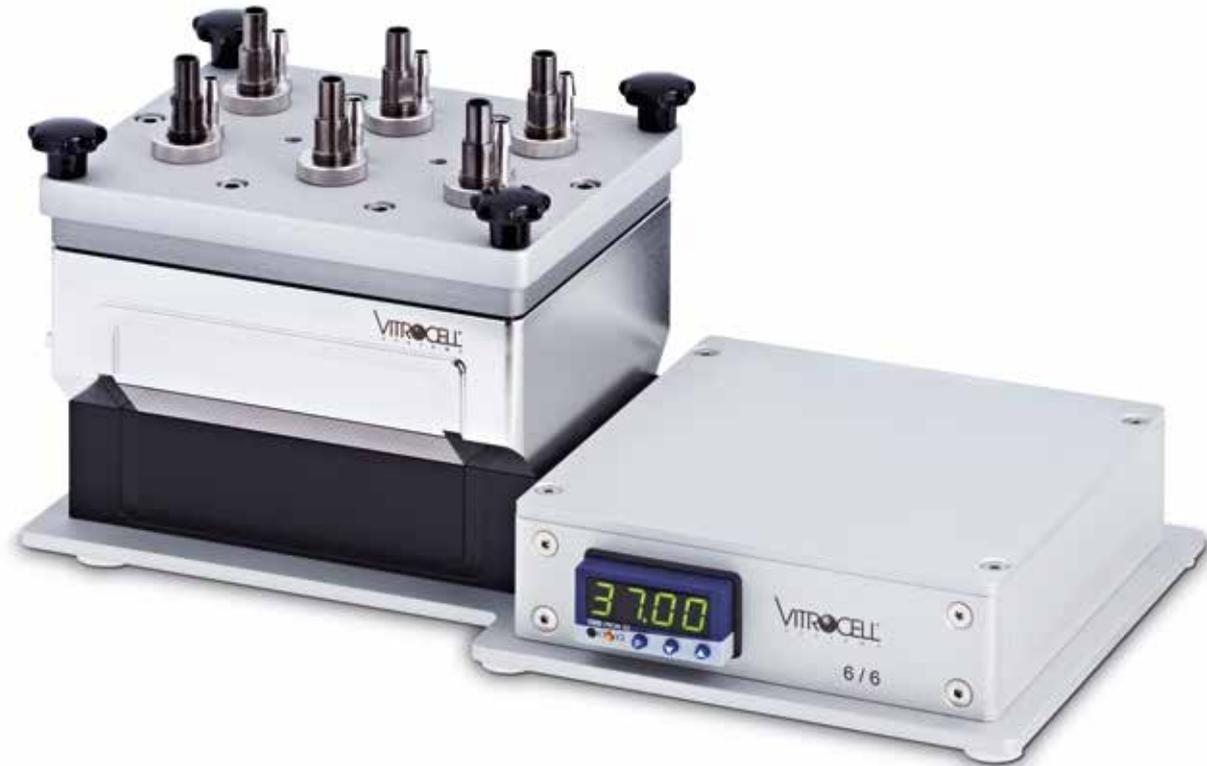
The VITROCELL® 6/6 module system has been specifically designed and engineered to facilitate the research of mammalian cell cultures in direct exposure to airborne substances such as gases, complex mixtures, nanoparticles and fibers. The system authentically simulates the conditions of human physiological exposure.
