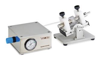
This automated solution is designed to press the button in a precise manner and synchronized with the puff regime. The trigger function is controlled by the software of the smoking machine.
