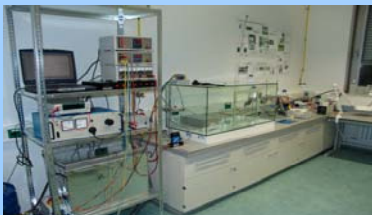
Fig. 4. The FA atmosphere was generated in a generation chamber using a static technique. Liquid FA was introduced in the chamber and vaporized. The gaseous FA was diluted with clean air to obtain concentrations of FA of 6.25, 12.5, 25, 50, 100 and 250 mg/m 3 .
