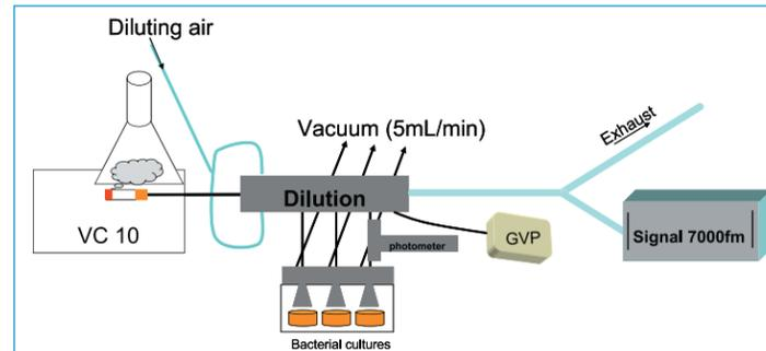
Figure 1. Schematic diagram of equipment set up.
