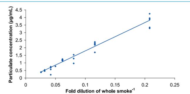
Figure 2. Smoke particulate concentration vs. smoke dilution.
