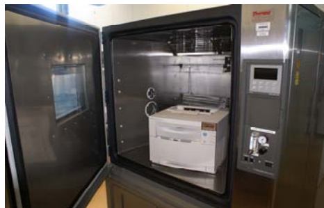
Fig 1: The emission test chamber with an investigated laser printer.
