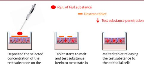
Figure 1 : Principle of exposure with the Dextran tablet (Huang et al., 2012)
