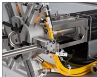
Powerful syringe drive by linear motor
