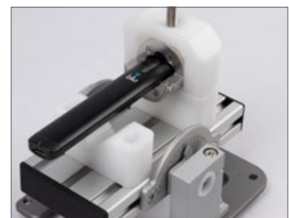
Standardized holder system for ENDS products
