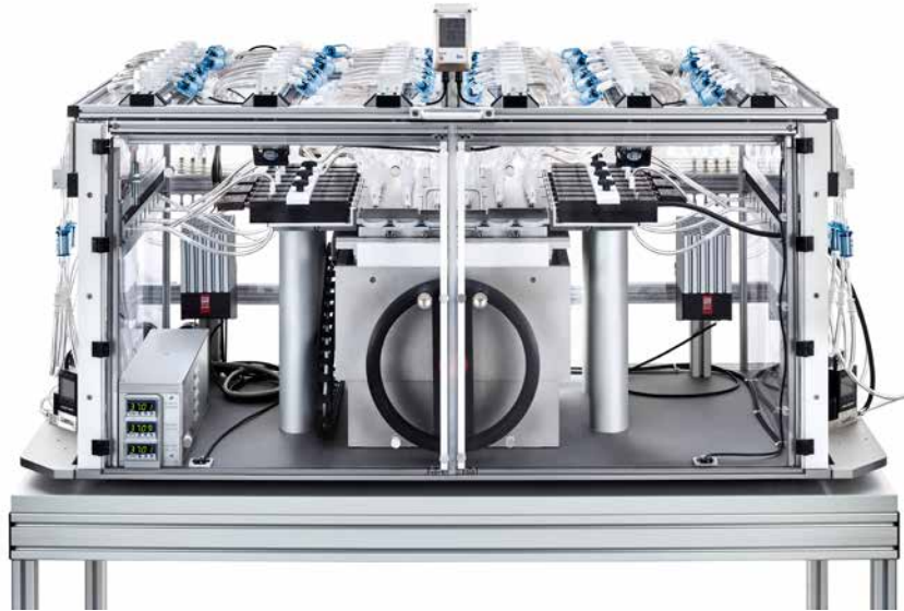
The entire system with integrated humidification system is housed in a climatic chamber.
