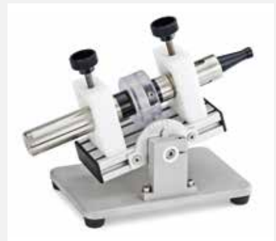
The system consists of Vapestart Controller, e-cigarette holder and different Vapestarter units.
