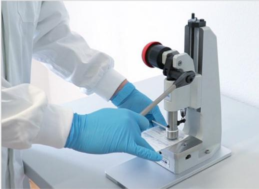
The procedure is as follows: place the skin sample on the ground plate, push the lever of the press downwards and punch into the skin. Then move the cutting tool in a circular manner to finalize a precise cut. Remove the sample.
