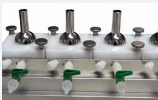
The receptor fluid can be sampled by using practical quarter-turn valves.
