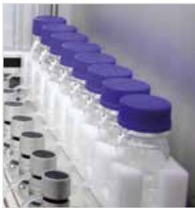
1 | Receptor fluid is stored in glass bottles and can be supplied gravimetrically or by syringe to the VITROCELL® Skin Exposure Module.
