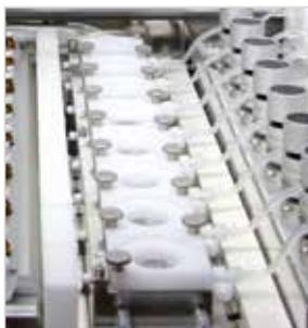
2 | The VITROCELL® Skin Exposure Module has an 8 chamber capacity and an integrated water bath heating circuit (e. g. 32-34 °C). Magnetic stirrers enable receptor-fluid agitation at variable rates.
