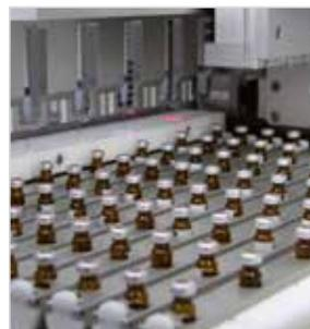
4 | The samples are delivered to an arrangement of 10 vial magazines each containing 8 vials. The magazines can be cooled (e. g. 5 °C).
