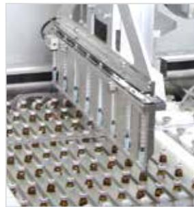
3 | A linear arrangement of up to 8 stepper-motor controlled individual syringes ensures precise sampling and highly reproducible results.
