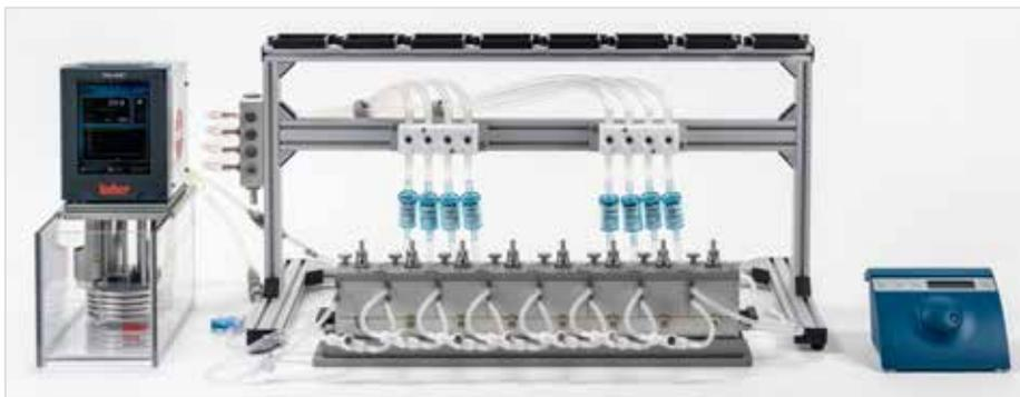
Base module incl. covers, 8 magnetic stirrers, stirrer control unit and water bath.
