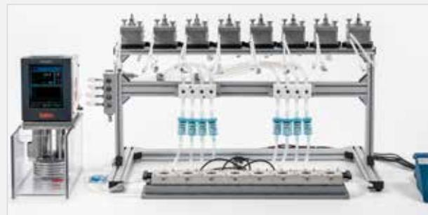
Skin Aerosol Max with 8 individual Aerosol Exposure Tops and their respective holders on the rack.
