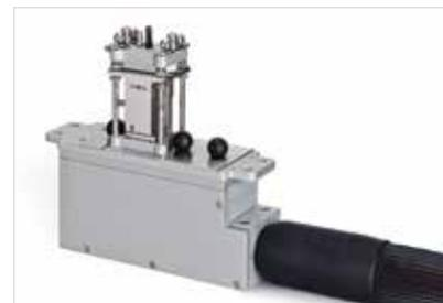
Unique flexible heated transfer line and customized sampling solution for the VITROCELL® exposure module.
