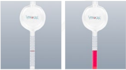
The drop of fluid in mm/60 s from the setpoint mark indicates the leakage rate.
