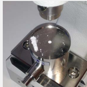
3 | Remove surplus powder from the press surface with a cell scraper
