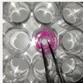
7 | Place the tablet on the apical surface
