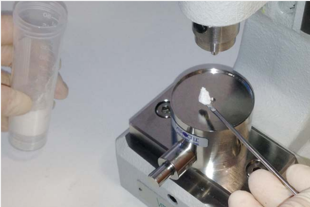
1 | Add Dextran powder to the press
