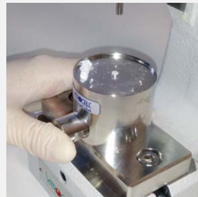
5 | Push the button to expel the tablet
