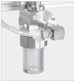
Small reservoir for recirculated flow mode
