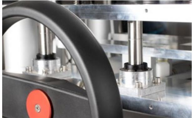
Heavy duty column guided lifting-closing mechanism for precise dosing
