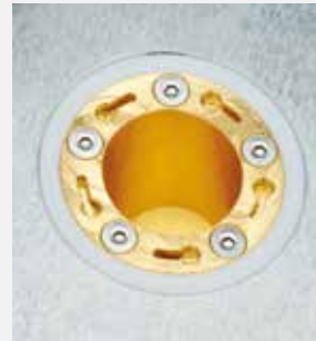
Optional microbalance sensor for dose monitoring
